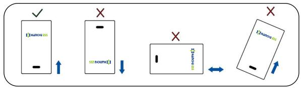
Figure 5 Installation Angle
