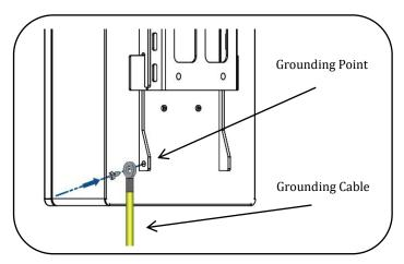
Figure 14 Sample of Battery Ground Connection
