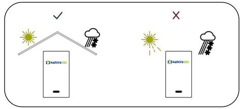
Figure 4 Installation Environment
