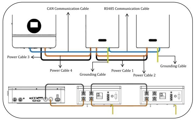
Figure 12 System General Wiring Diagram
