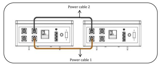
Figure 15 Sample of Power Connections Between Batteries
