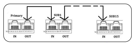
Figure 18 Sample of Communication Parallel
