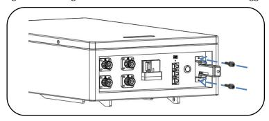
Figure 20 Logger Installation Schematic
