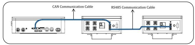
Figure 17 Sample of Connection for the Communication Cable
