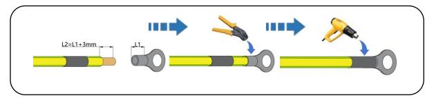
Figure 13 Sample of crimping method
